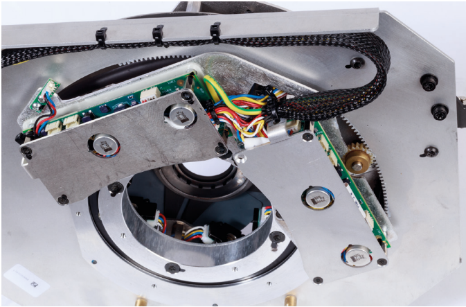
Aperture slide module with a deep opening for retracting the focus lens system, the pinion for rotating the aperture slide arrangement can be clearly seen on the right
