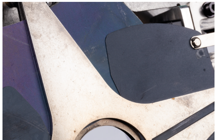
Aperture slider angled at the edge so that the opposite sliders on the same level can be angled more towards each other
