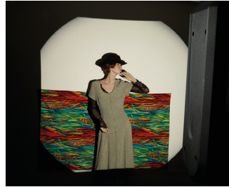
Four aperture slides slightly retracted and focused, showing the focus distance to the unaffected light cone
