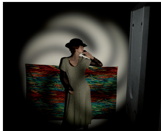
Frost 1 fully retracted zoom to 200 dec., focused on gobo
